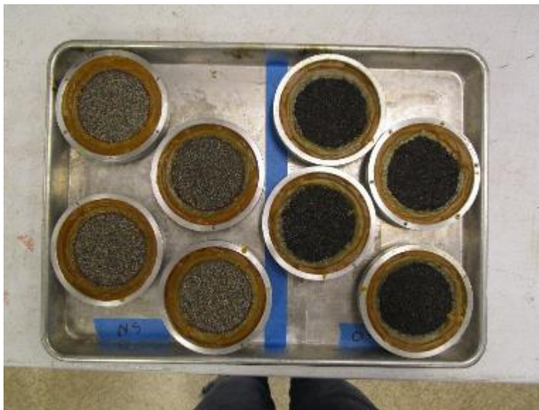
Photo No. 4 ASTM E96 Water Vapor Transmission - Specimen Assemblies
